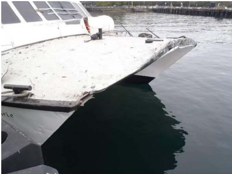
(Photo shows damage to the bow of the RACHEL MARIE as a result of the allision.)
